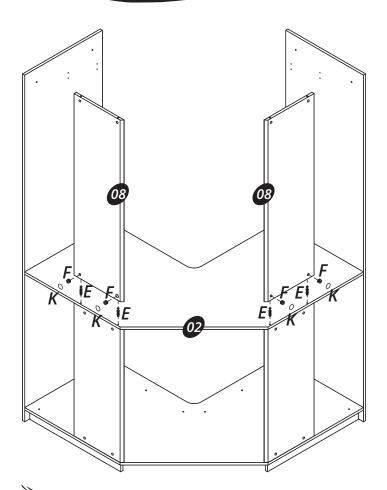
Connect the part (08) onto the part (02) with the hardware (E + F) Apply the hardware (K) on the hardware (F).
