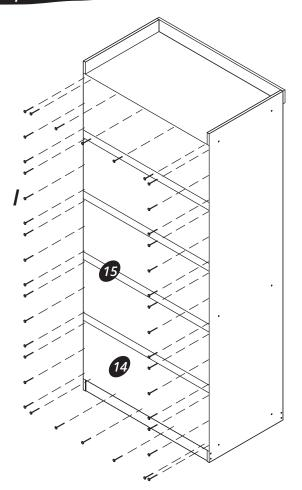
Connect all the parts (14) joining with the part (15) and the hardware (I).
