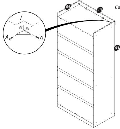
Connect the part (13) onto the part (03) and the part (04) joining the corners with the hardware (J) with the hardware (A).
