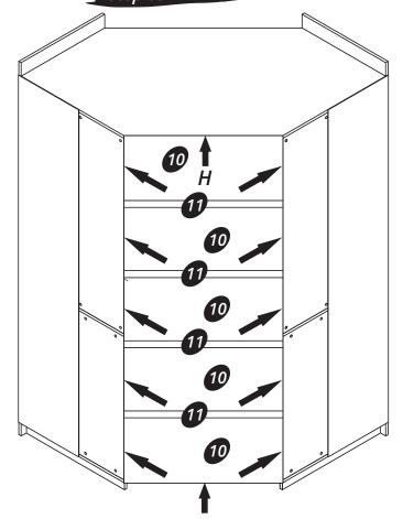
Connect the part (10) with the part (11) and the hardware (H).
