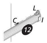
Fix the hardware (L) onto the hardware (I) with the hardware (C) after install the part (12).
