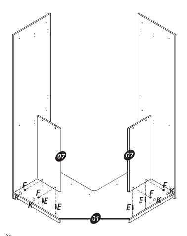
Connect the part (07) onto the part (01) with the hardware (E + F) Apply the hardware (K) on the hardware (F).
